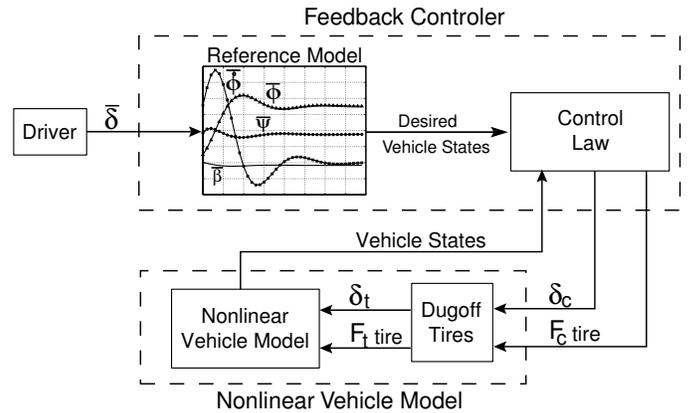
Figure 3. Block diagram of proposed control and simulation structure
