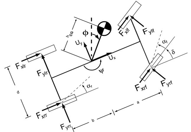
Figure 1. 4 wheel vehicle model with roll
