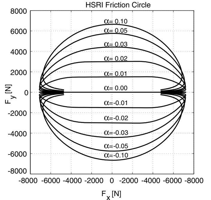
Figure 2. HSRI tire model friction circle
