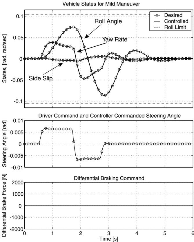
Figure 5. State evolution during normal maneuver
