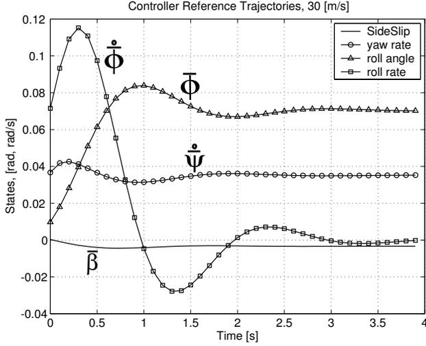
Figure 4. Example of reference trajectories given an input steering angle and some initial condition
